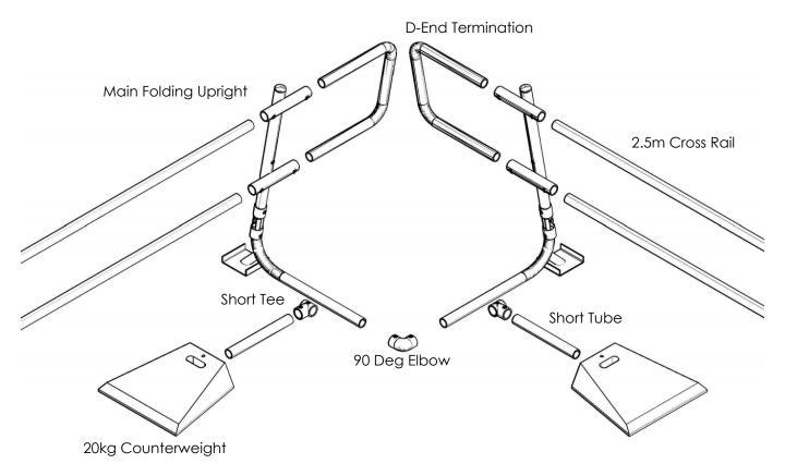
Begin by assembling a complete corner unit consisting of two folding uprights, two counterweights, two d end terminations, two short tee's and a 90 deg elbow.
