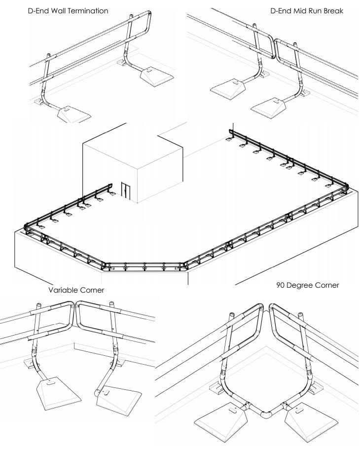
**Configuration** Free Standing Folding Edge Protection - System Configuration
